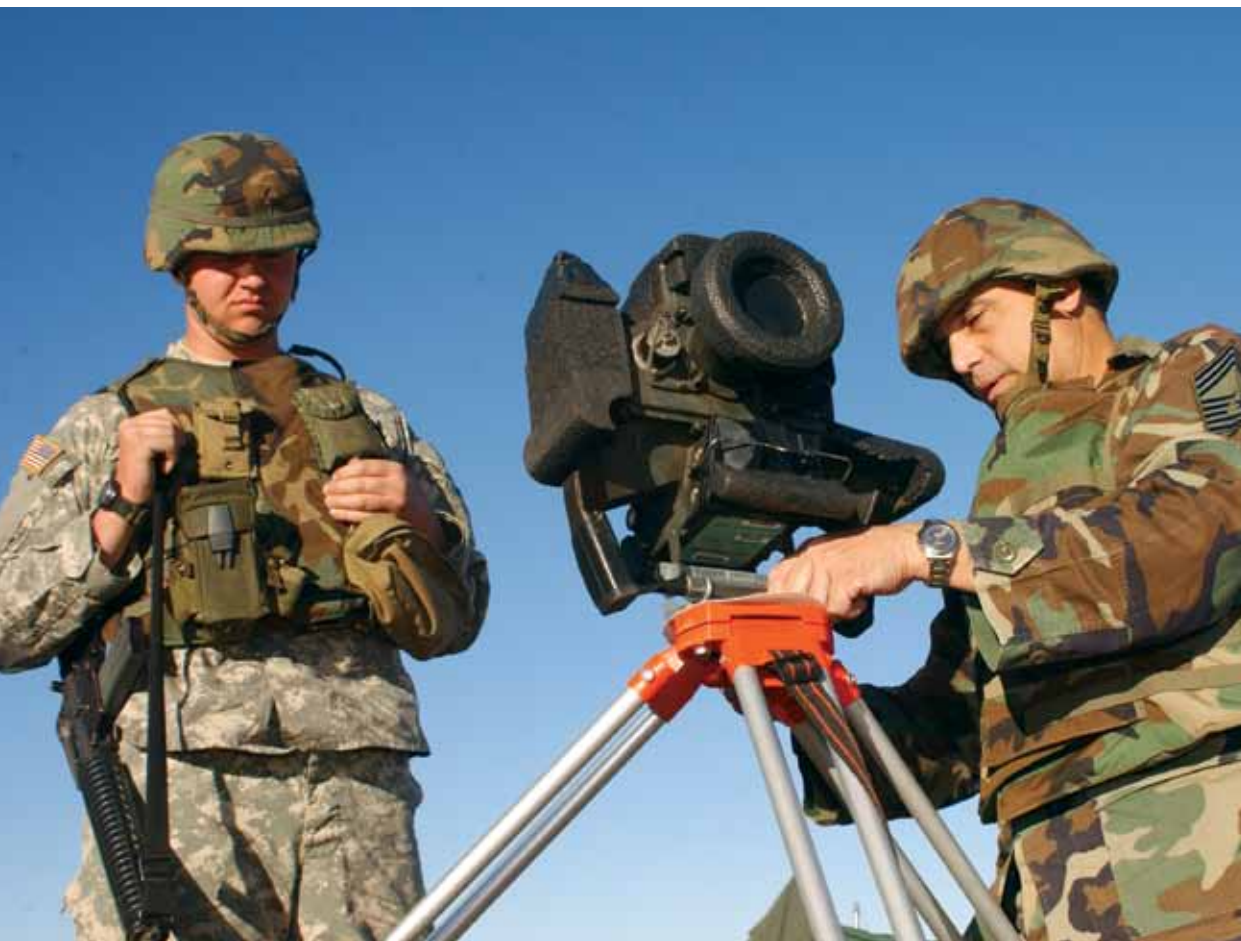
Guardsmen often innovate new methods, such as adapting a photography tripod to hold the heavy night-vision scopes employed by the Border Patrol. Here, an Air Guard member makes final adjustments on a tripod mount. OJS Public Affairs Office, JTF-AZ
